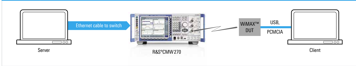
FIG 4 Test setup for data throughput measurements with the R&S®CMW270 WiMAX™ communication tester.
