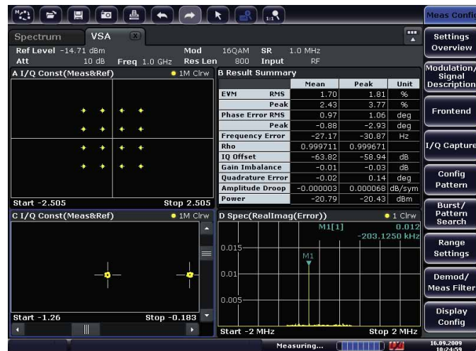
FIG 4 Four measurement windows that can be displayed simultaneously provide a comprehensive overview. In this measurement example, the zoomed constellation diagram and the spectrum of the error vector point to a sinusoidal interferer as cause of the increased EVM value.
