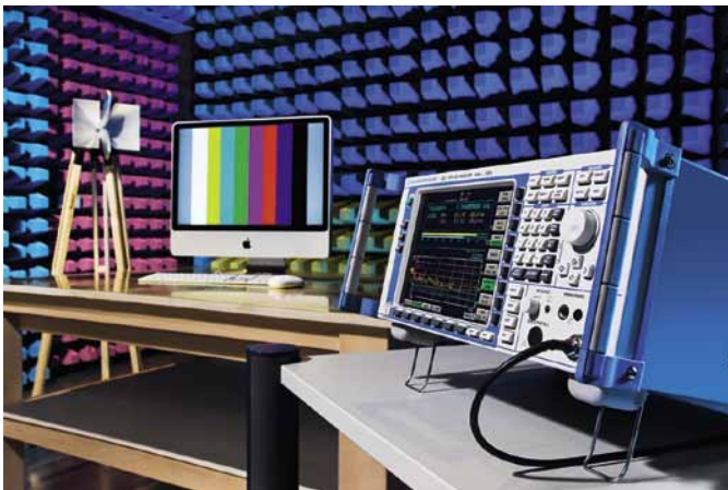
FIG 1 Measurement of radiated disturbance in line with the product standard CISPR 22:2005/A1:2005/EN 55022:2006/A1:2007 for IT equipment in the range from 1 GHz to max. 6 GHz using the R&S®ESCI7 EMI test receiver and the R&S®HF907 double-ridged waveguide horn antenna.
