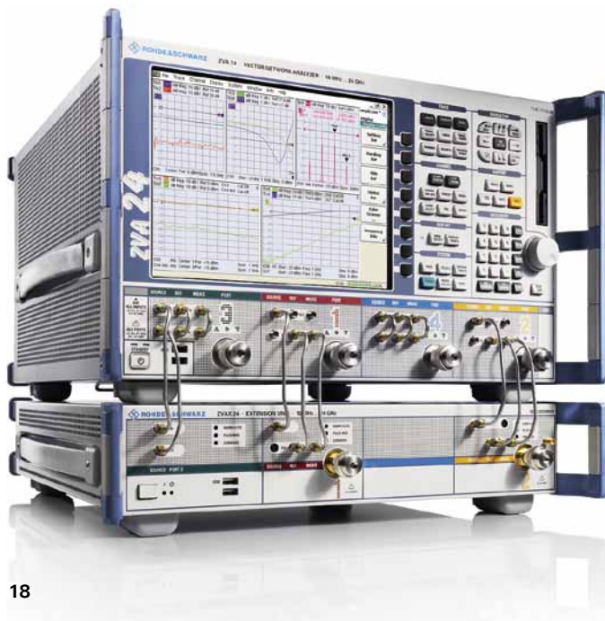
FIG 1 Connecting the R&S®ZVAX24 extension unit to the network analyzer is easy: The extension unit is placed under the network analyzer, and the RF ports of the two units are connected by means of semi-rigid cables. The extension unit is controlled via USB directly from the network analyzer.
