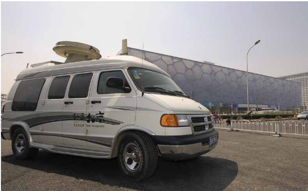
FIG 1 Rohde & Schwarz mobile direction finders supported the fixed systems from test vehicles.
