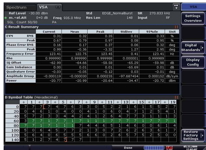
FIG 7 Tabular overview of the measured modulation parameters and display of the bit stream.
