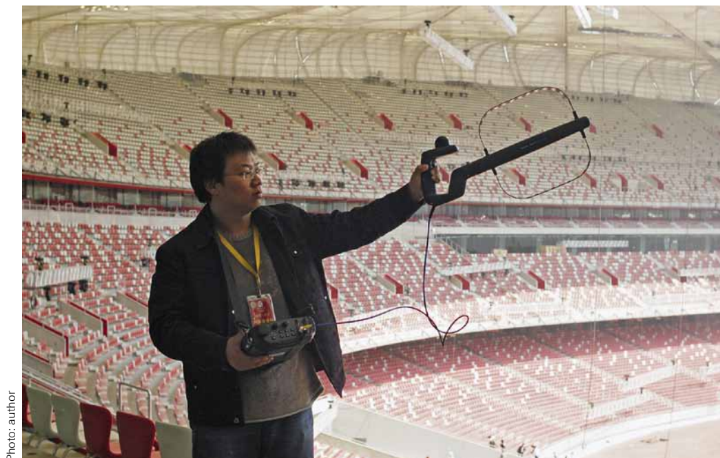
FIG 2 The R&S®PR100 portable receiver and R&S®HE300 directional antenna modules help to trace interfering signals quickly and efficiently.
